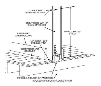
Figure 1. Routing Thermostat Wires
